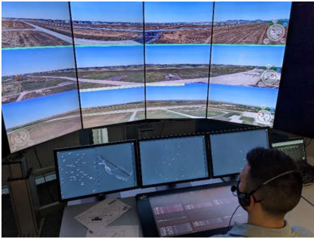
Figure 4. Multiple remote tower and ground environment at DLR Braunschweig's Remote Tower Lab (LIT).
